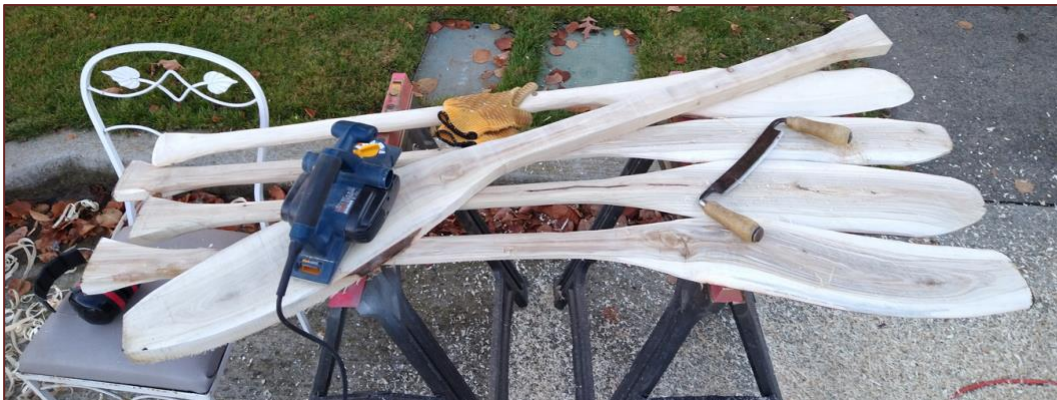
Blue electric power planer used to shave knotty areas which are almost impossible to carve with a drawknife. Its use greatly sped up the bulk paddle production.
