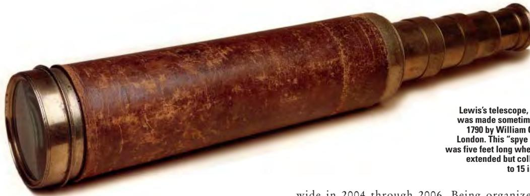
Lewis's telescope, which was made sometime after 1790 by William Cary of London. This "spy glass" was five feet long when fully extended but collapsed to 15 inches.
